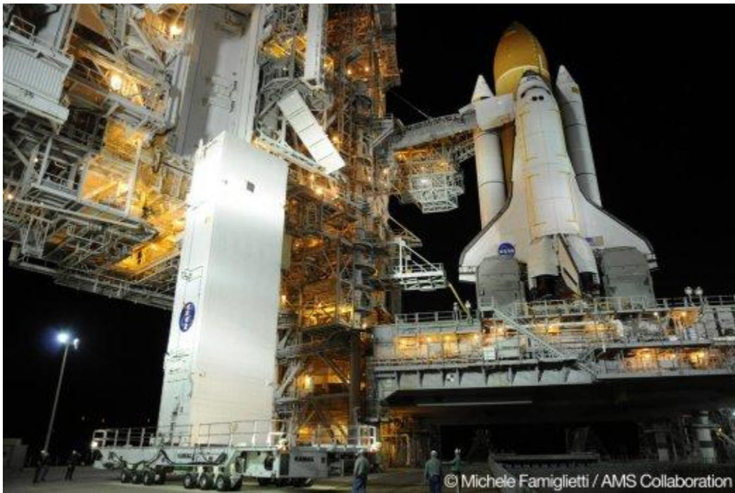
Alpha Magnetic Spectrometer With Endeavour: The AMS canister is prepared for loading into the cargo bay of space shuttle Endeavour. Michele Famiglietti/AMS-02 Collaboration
