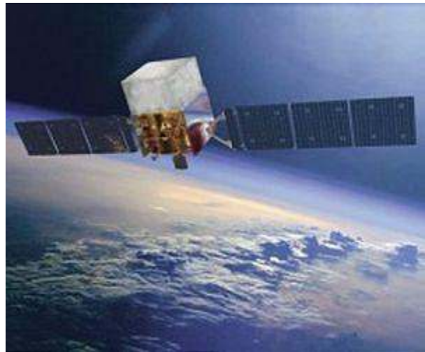
The Fermi Gamma-ray Space Telescope detects gamma-rays by tracking the electrons and positrons they produce after striking layers of tungsten. (Credit:NASA/Goddard Space Flight Center Conceptual Image Lab)
