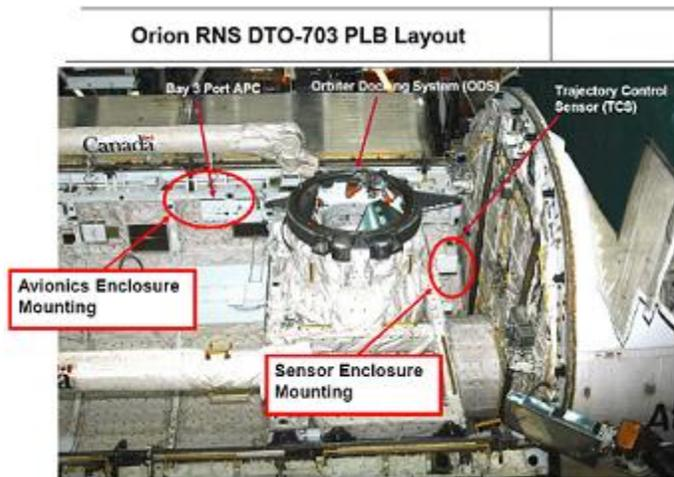
Finally, the Orion Rel-Nav Sensor (DTO 703) will be mounted on the Orbiter Docking System (ODS) in Trajectory Control Sensor slot 1 and on an Adaptive Payload Carrier in bay 3 port of the Payload Bay.
