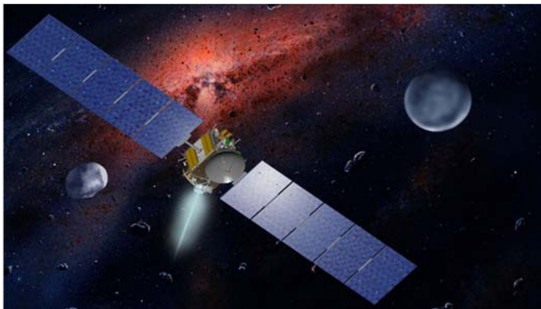
ASTEROID SEEKER: NASA's Dawn spacecraft, shown in an artist's concept, is propelled by ion engines. The satellite will study asteroids to help understand how planets form. (Illustration: NASA)
